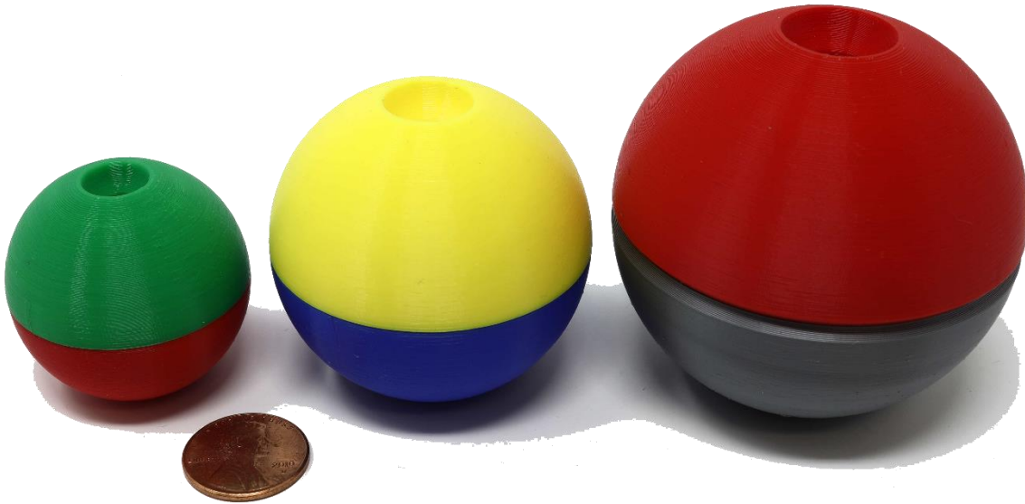
Figure 6: Three sizes of 3D printed flippe tops. The largest one has an equatorial groove for a string.
